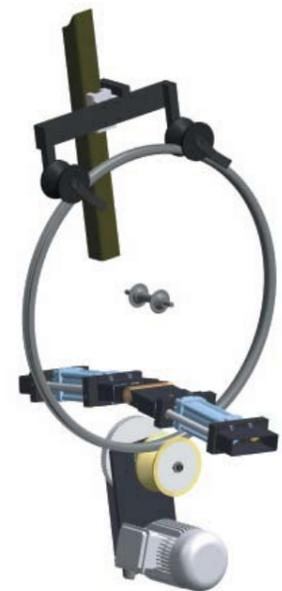
**For some types** of wheels it may be advantageous to stabilize the laced wheel before it is trued. In the Holland Mechanics Stabilizer two cylindrically-shaped cushions push the spoke screen just to a preset flexibility limit to make them more compliant when truing. The stabilizer works well with 36-spoke wheels, but equally with 14-spoke wheels.
