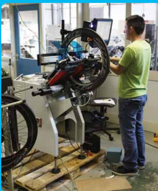
rim with the risk of breaking it and you are certain that the rim has moved the pre-set millimetres ensuring the spoke de-winding has taken place.
